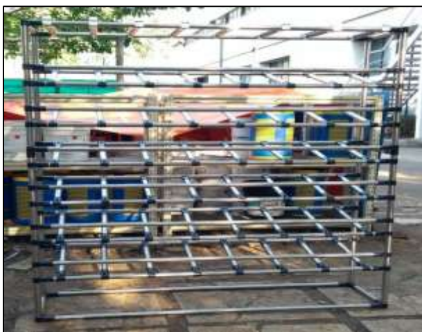
Pipe Storage Rack
