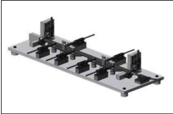
Welding Jig Fixtures
