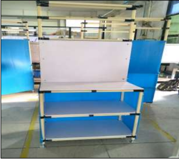
Work Table in pipe & Joints
