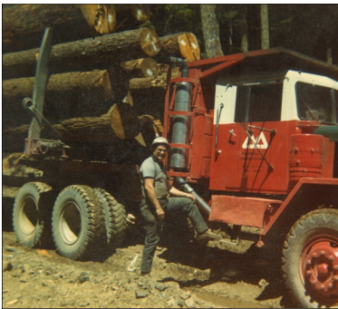
Alex Spencer (circa 1970) with 1958 "Hayes" HD "H-41" Sproat Lake with V-8 GMC engine.
