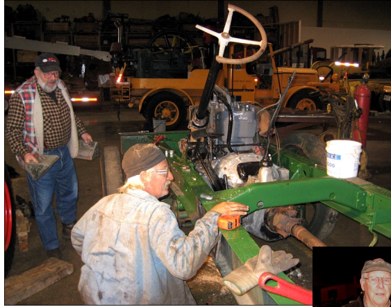
(left) With the engine now mounted, Les eyeballs the frame before welding new brackets on. (Note Vic holding the brackets) (below) John & Les Stevens with the steering wheel, before its restoration.
