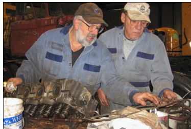
Vic Laughlin (l.) and Frank Anderson work on the head of the engine for the '65 'Mercury'. (We regret to say that Frank died suddenly in December. He will be missed.) (below) Engine being lowered into place.
