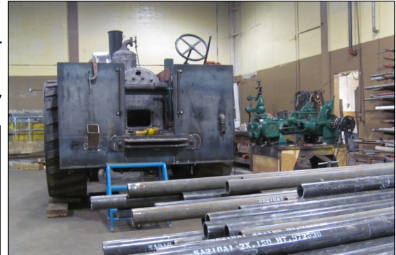
Boiler tubes , awaiting installation. Newly-fabricated Operator's deck & water tank visible. (below) Boilermakers rolling tubes Brent Pennington (l.) & Barry Dobrensky. Bill Rogers and Leon McCrea also worked on it.
