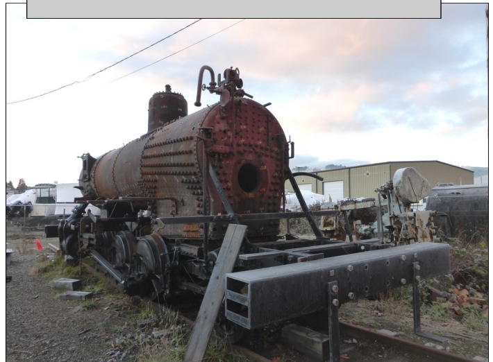
Work on the 1923 “Baldwin” - CANFOR ‘112’ Work progresses slowly on the loci collected from Beaver Cove in 2015. Above, the Brake cylinders are being re-installed after restoration. Below, a new rear bumper has been fabricated for under the cab. The pony wheels/front axle assembly have been straightened and will be re-installed this spring.
