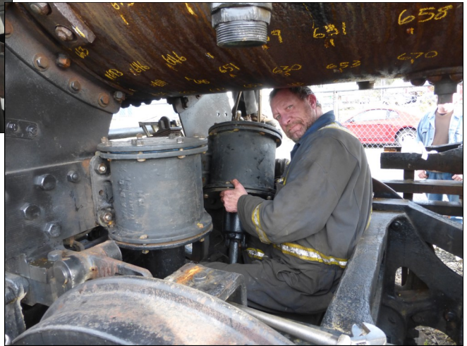
Work on the 1923 “Baldwin” - CANFOR ‘112’ Work progresses slowly on the loci collected from Beaver Cove in 2015. Above, the Brake cylinders are being re-installed after restoration. Below, a new rear bumper has been fabricated for under the cab. The pony wheels/front axle assembly have been straightened and will be re-installed this spring.
