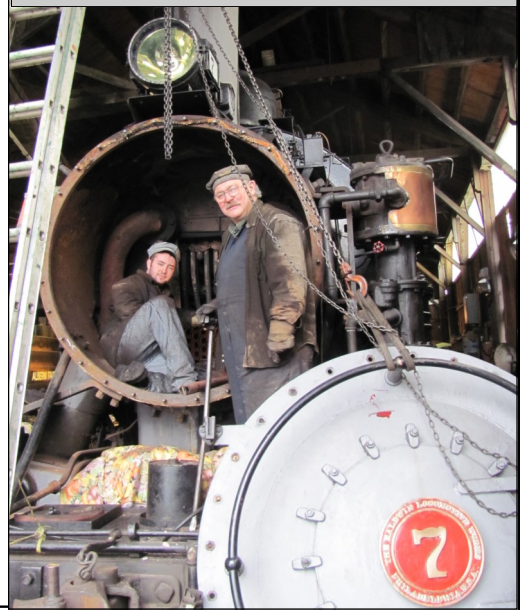
(Below) Dan & Rod working in the smoke- box of "Number Seven".
