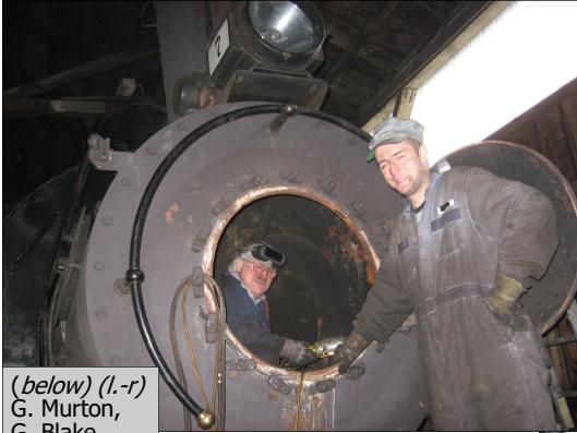
(left) In the 'Smokebox' Dan (l.) and Rod Gledhill work on the bracket holding the air pumps to "Number 7".
