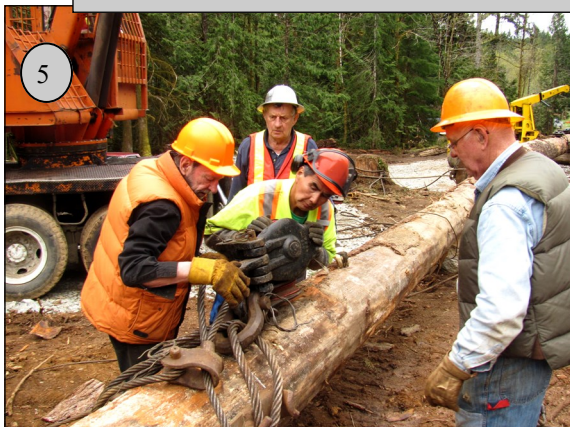
6. Blocks & lines ready for the lift.
