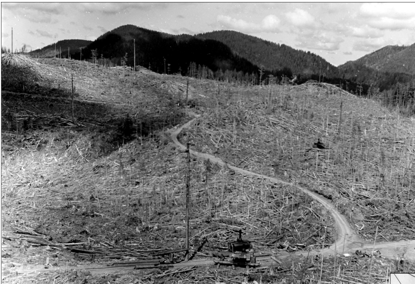
(above) HOW MANY SPAR TREES can you see? Note the ‘home tree’ with a skidder in the foreground. Piles of logs may be seen at the foot of ‘cold deck’ trees. Eg. Top left corner. This is near Holberg.
