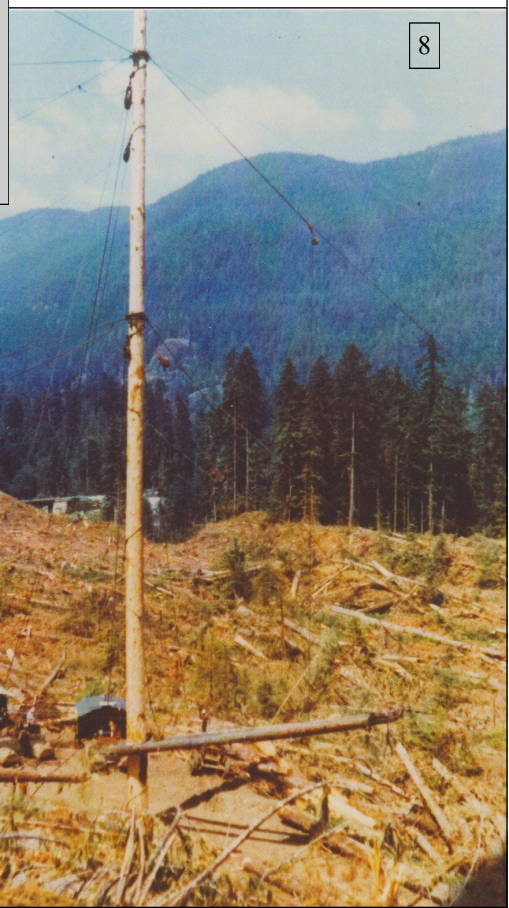
#8: A Heel boom has now been rigged and the tree is about ready to work. Notice the loading and yarding donkeys at the foot of the tree—the same layout as at the McLean Mill Show.
