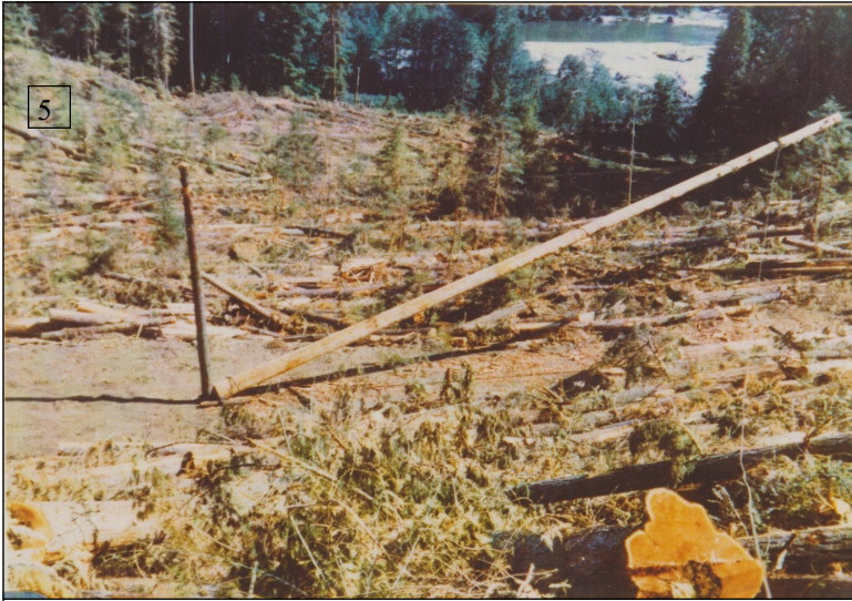
#5: With the Gin-pole up, now it is time to raise the spar. (This was known as the "Flying Gin pole" because, as you see in #6, with the spar past 45 degrees, the gin pole's job is done and it is now hanging in the air.)
