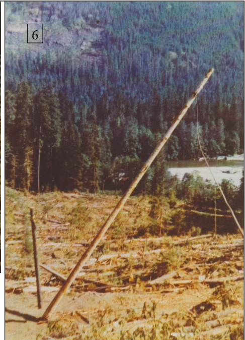
#5: With the Gin-pole up, now it is time to raise the spar. (This was known as the "Flying Gin pole" because, as you see in #6, with the spar past 45 degrees, the gin pole's job is done and it is now hanging in the air.)
