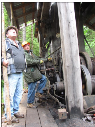
Jack on the levers of the yarder, brings in a 'turn'.
