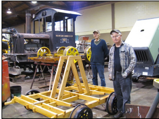
(left) The new Handcar Matt Gregory (r.) and J. Jansma built the car this winter and put it on the rails in September.
