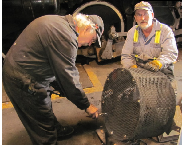
3 Dan Gledhill & Ted Mollet repair "No. 7"'s spark arrester.
