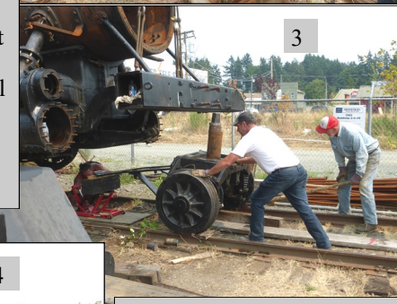
Photo 3: Rolling the axle under the frame. (Steve Alder & Harold Carlson.) Steve is with the Vancouver Island Model Engineers' club in Victoria and was a surprise visitor.
