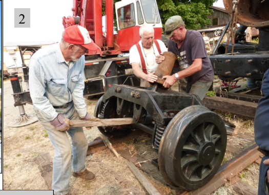
Photo 2: Installing the pin which links the front axle to the main frame. Harold Carlson, Michael Stewart and Big Steve wrestle the pin into place.
