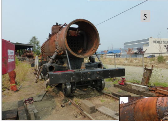
Photo 5: It is now a "2-6-2" locomotive again. The Roundhouse is visible behind the locomotive. The plan is to move the '112' under cover in the Roundhouse this winter.
