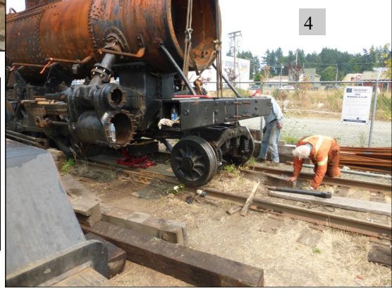
Photo 5: It is now a "2-6-2" locomotive again. The Roundhouse is visible behind the locomotive. The plan is to move the '112' under cover in the Roundhouse this winter.
