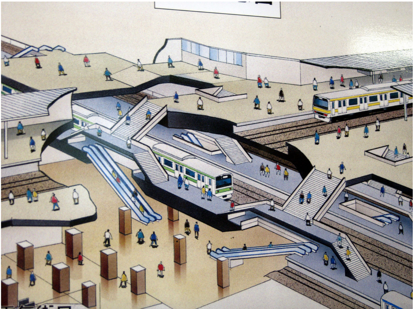
Figure 1: Underground rail station with multiple train platforms
