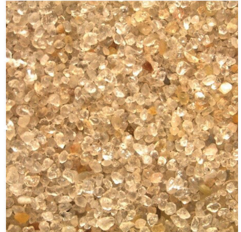
SQS 100m standard sand suits technical and economic requirements for wells with normal closure stress.
